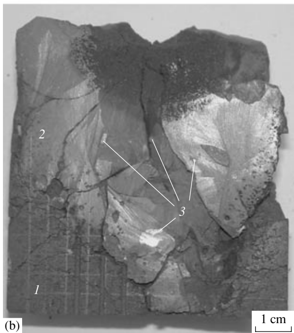
Fig. 4. Axial cross sections of oxide ingots and SM samples: (a) SACR-8 experiment, (b) SACR-9 experiment; (1) SM sample, (2) oxide melt, (3) metallic inclusions, (4) epoxy resin.
